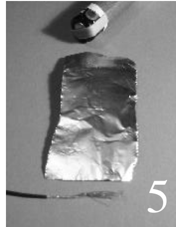
5. The wire should be stripped so that the bare end is about an inch long.
